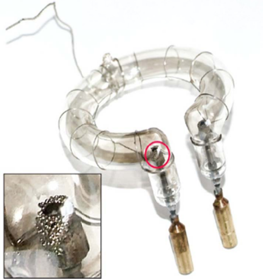
Broken Flash Tube
